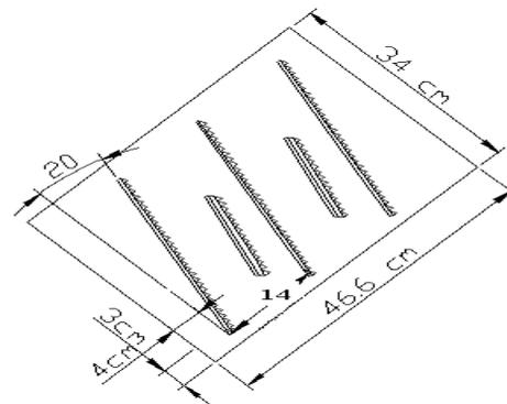
Figure 12: Fin distribution on condenser surface
