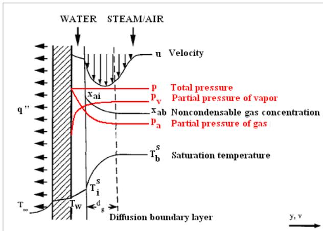
Figure 2: Schematic illustration of condensation with non-condensable gas.
