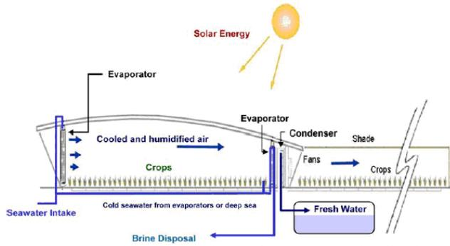
Figure 1: Schematics of green house for sea water desalination [4].
