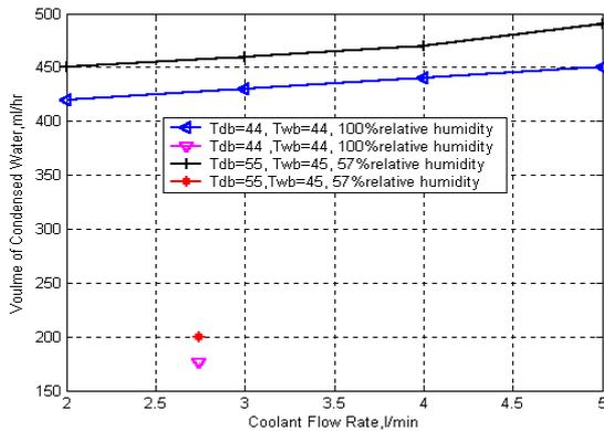
Figure 13. Comparison of produced condensate water (ml/hr) for the vibrating plastic surface condenser-II (water flow rate of 2.74 ml/min) and flat plate channel condenser at air velocity of 0.4 m/s and constant coolant temperature of 15° C
