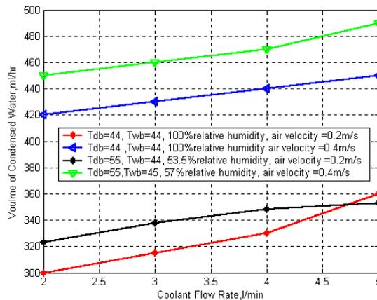
Figure 11: Variation of water condensate by varying the air speed at constant coolant temperature of 15 °C
