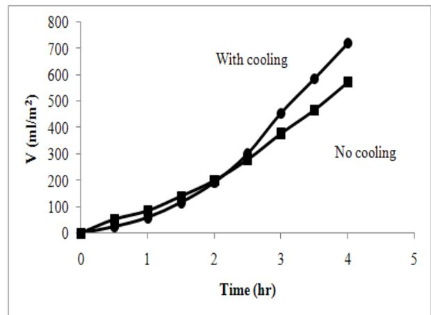
Fig. 6: Effect of cooling the glass cover on the productivity of the unit.
