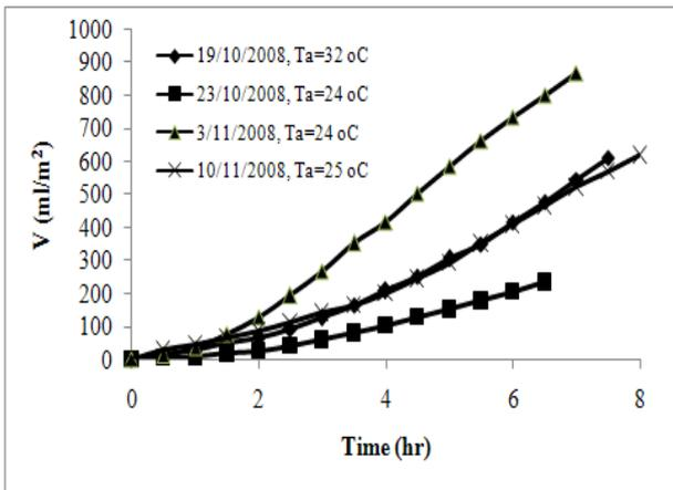
Fig. 4: Cumulative volume of desalinated water at different time of the year using jojoba oil as a thermal fluid.
