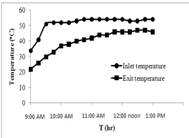
Fig. 8: The inlet and the exit thermal fluid (water) temperatures in the evaporator.
