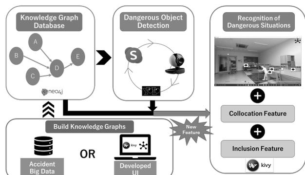
Fig. 2. System configuration for the detection of dangerous situations (Instructor’s PC)
