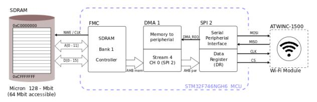
Fig. 5. Proposed hardware architecture for the wireless communication
