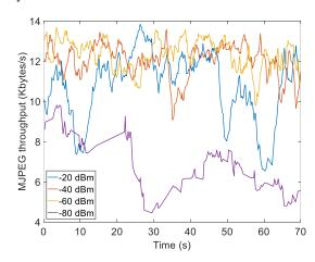
Fig. 8. MJPEG throughput for different wireless signal strengths
