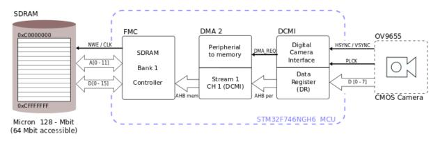
Fig. 4. Proposed hardware architecture for image acquisition
