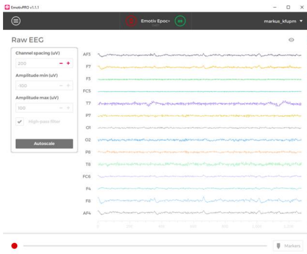
Fig. 11 Real time EEG readings corresponding to the raw data read by the 14 channels.
