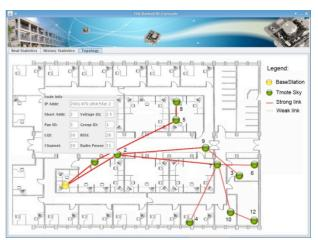
Figure 6. Snapshot of WSN topology using EMP GUI
