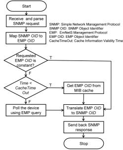
Figure 4. Device monitoring procedure from SNMP Manager
