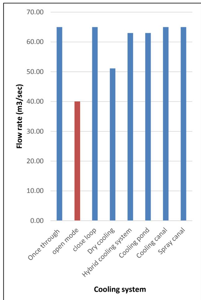
**Figure 9: Flow Rate Comparison**
