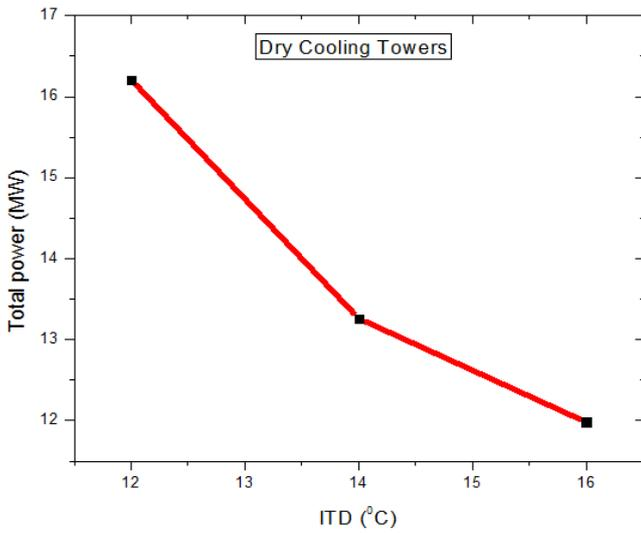
Figure 6: Dry cooling tower results
