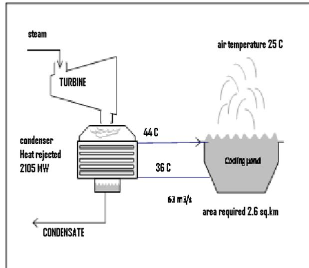
Figure 7: Results for cooling pond close loop
