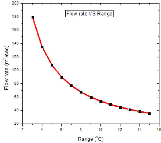
**Figure 2: Variation of Flow Rate with Condenser Range**
