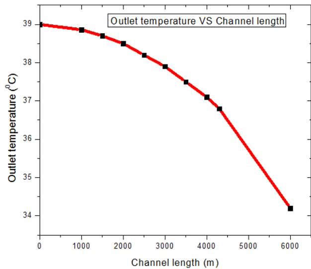
Figure 5: Variation of Outlet Temperature with Length of Channel
