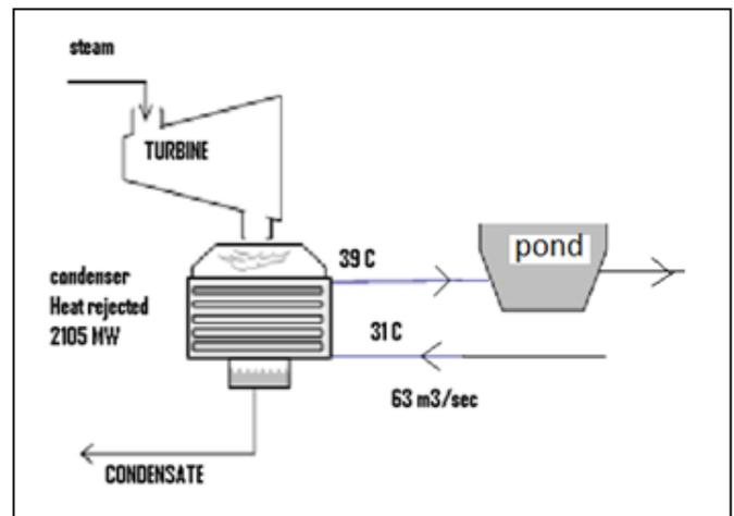
Figure 8: Once Through with Cooling Pond.
