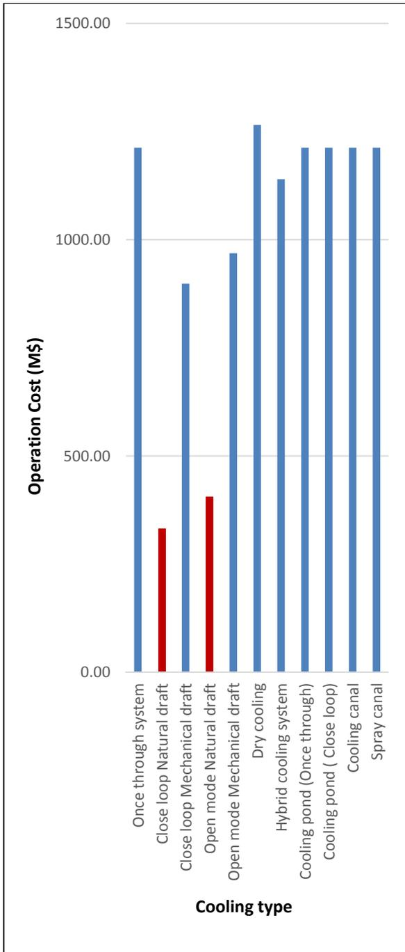
Figure 12: Operation Cost Comparison
