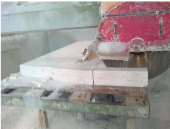
Figure 2: Fraiza during cutting stone slabs in one of Palestinian stone factories.
