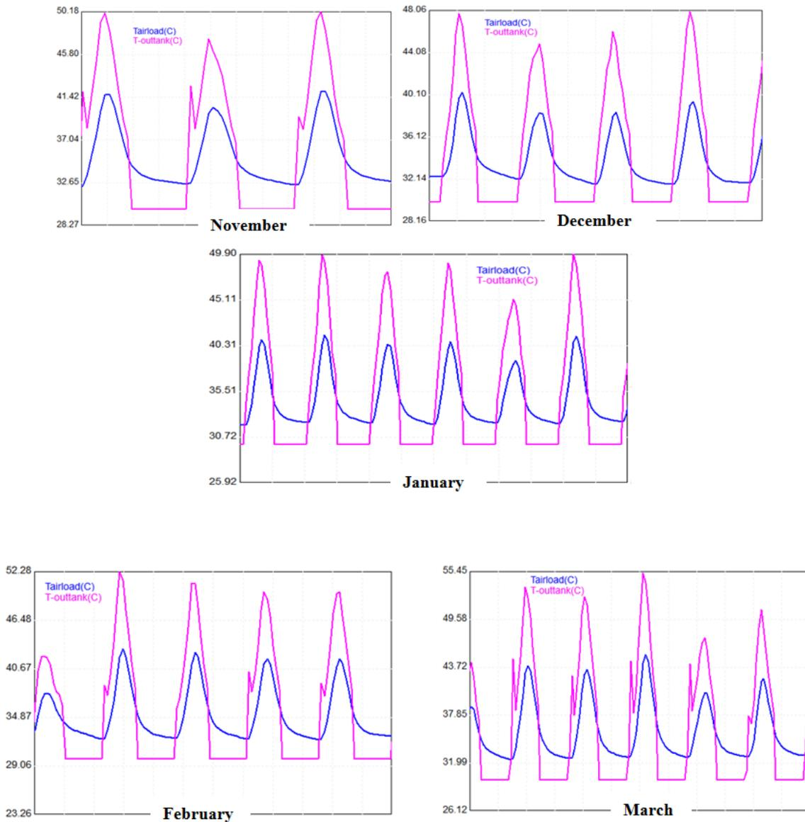
Fig. 5. Maximum hourly variations of tank outlet temperature and air load temperature
