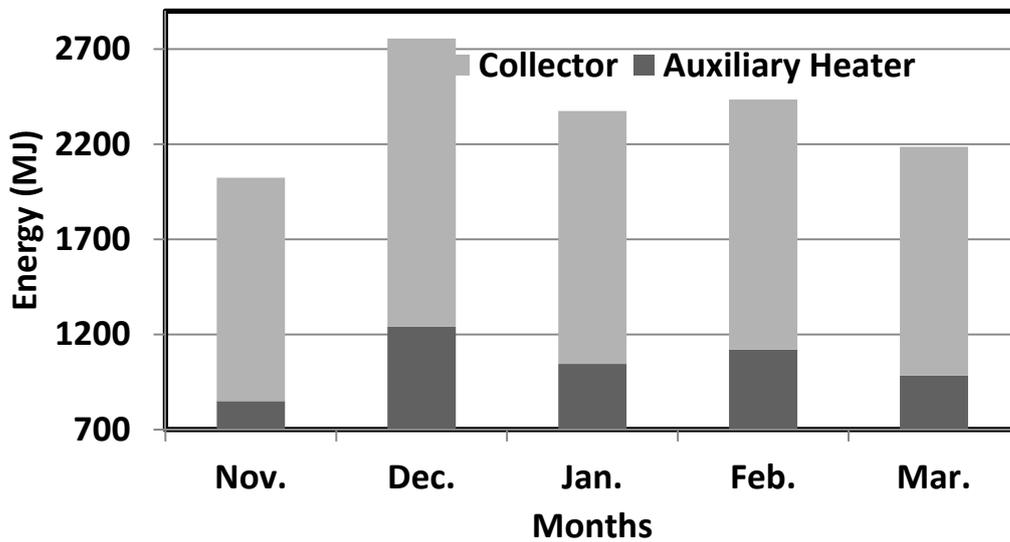
Fig. 7. Energy of solar collector and auxiliary heater
