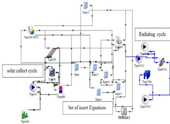
Fig.2 .The system represented in TRNSYS components
