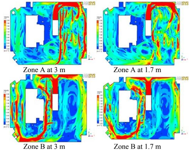
Figure 10: Velocity contours at 3 m and 1.7 m for zones A and B
