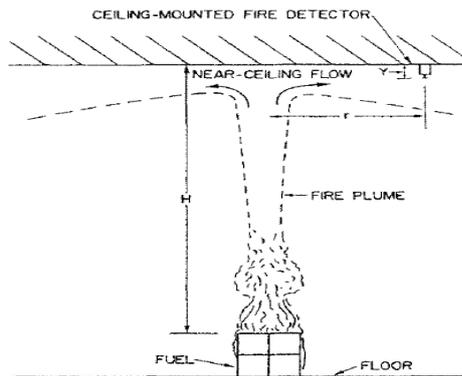
Figure 1: Ceiling jet flow beneath an unconfined ceiling [20]
