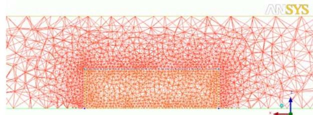
Figure 2: Volume mesh on x-z plane at y = 25 m
