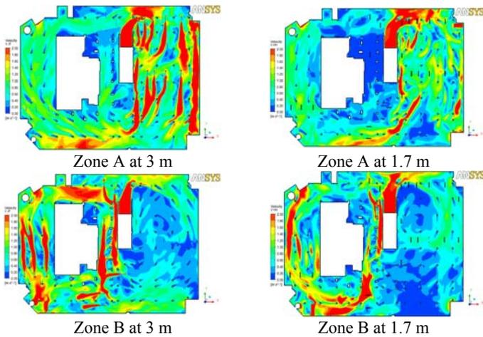
Figure 13: Velocity contours at 3 m and 1.7 m for zones A and B
