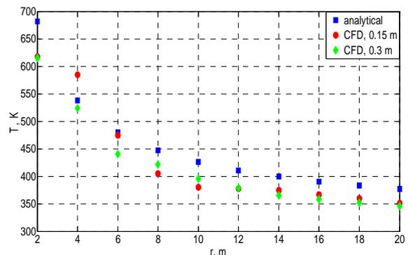
Figure 3: Ceiling temperature at different distances from fire center
