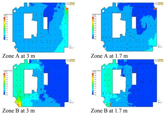
Figure 18: CO<sub>2</sub> mass fraction contours for zones A and B
