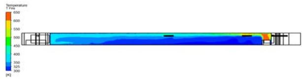
Figure 15: Temperature contour along y-axis, zone A
