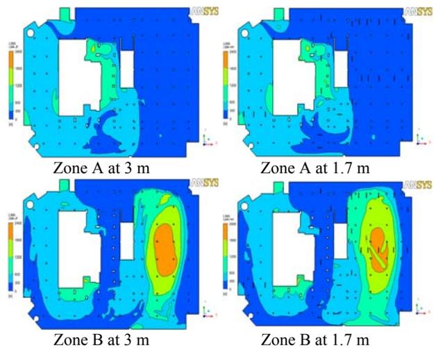
Figure 11: LMA contours at 3 m and 1.7 m for zones A and B
