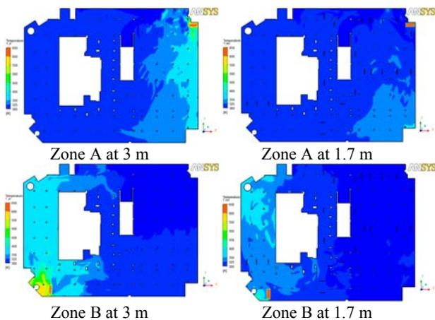
Figure 14: Temperature contours at 3 m and 1.7 m for zones A and B
