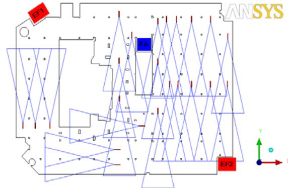
Figure 6: Configuration of the jet fans
