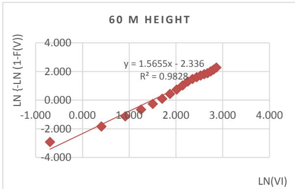
Fig. 2(a) Graphical method to estimate c & k at 60 m
