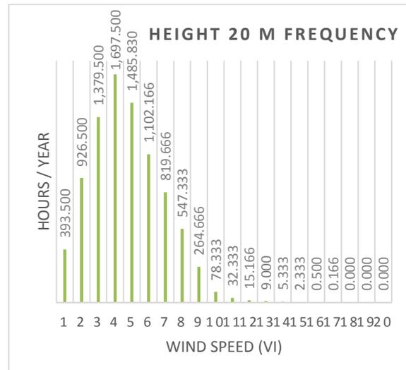
Fig. 1(c): Wind speed probability at 20 m height
