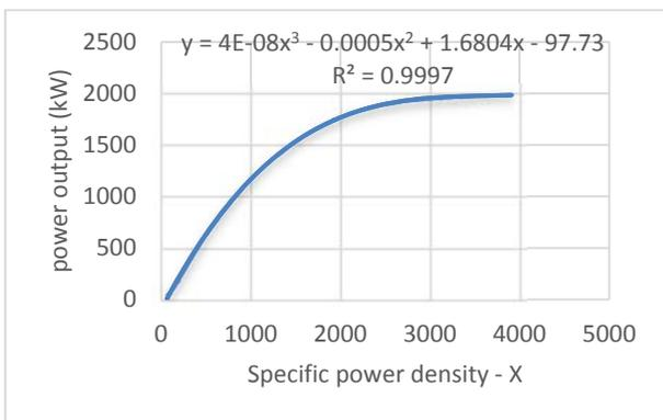
**Fig. 5: 3<sup>rd</sup> order relation between power and cubic wind speed**
