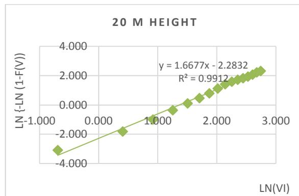
Fig. 2(b) Graphical method to estimate c & k at 20 m heights
