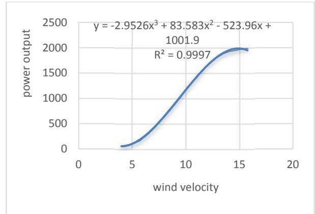
Fig. 4 The relationship between wind speed and power output between cut-in and rated speeds for V80-2.0 wind turbine
