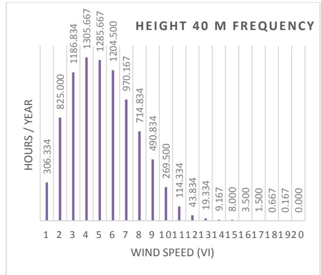
Fig. 1(b): Wind speed probability at 40 m height
