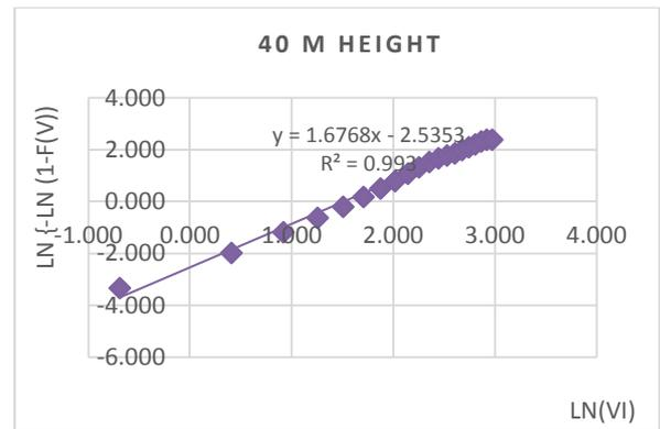
Fig. 2(c) Graphical method to estimate c & k at 40 m height
