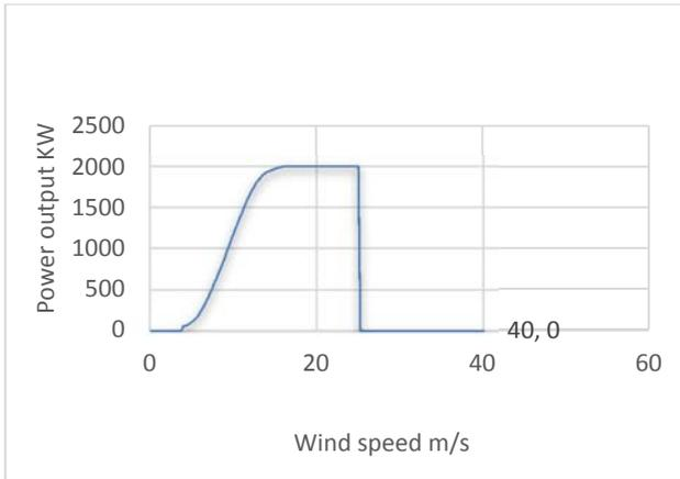
Fig. 3 Power curve for Vestas V80-2.0
