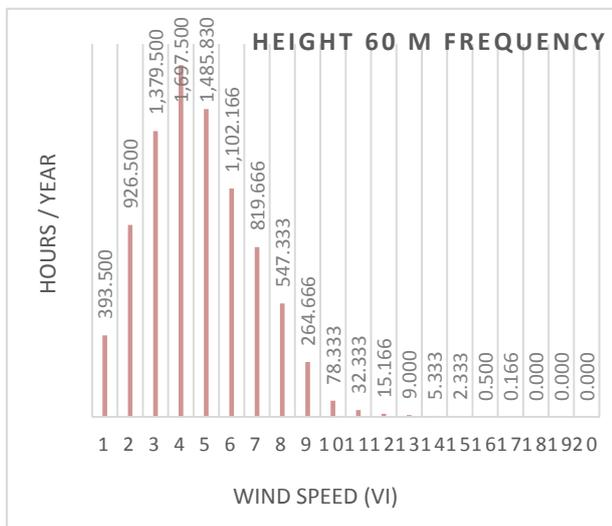
Fig. 1(a): Wind speed probability at 60m height
