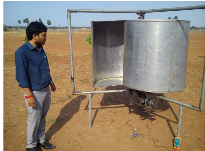
Figure-1. : Savonius Vertical Axis Wind Turbine at DBSIT, Kavali, SPSR Nellore District, AP.
