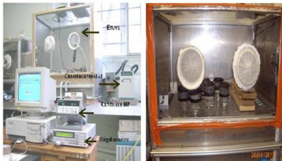
Fig. 1. Equipment and dryer at the controlled atmosphere
