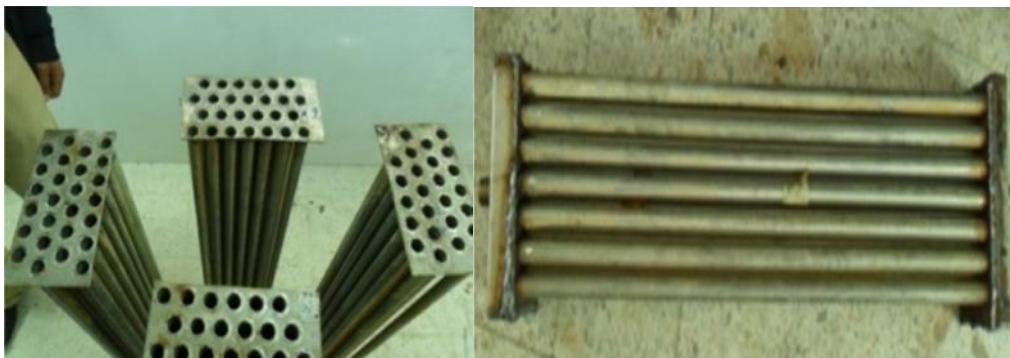
Figure 4: The stainless steel heat exchangers
