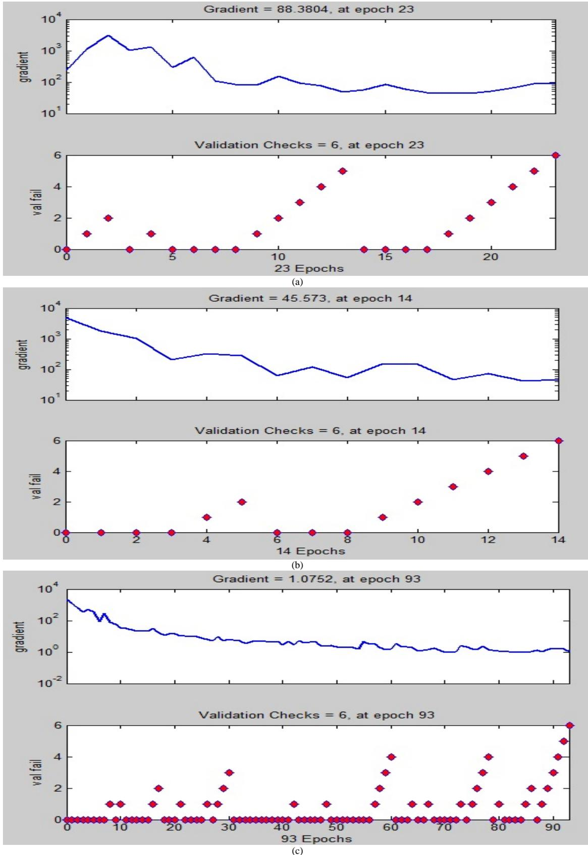
Figure 3: The variation of gradient error, and validation checks to a) Elman Network b) NARX Network c) Feedforward Network.
