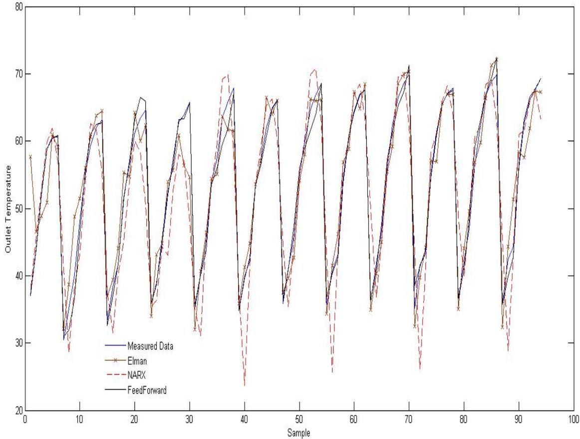
Figure 5: Comparison between experimental and estimated outlet temperature of the thermal energy storage.
