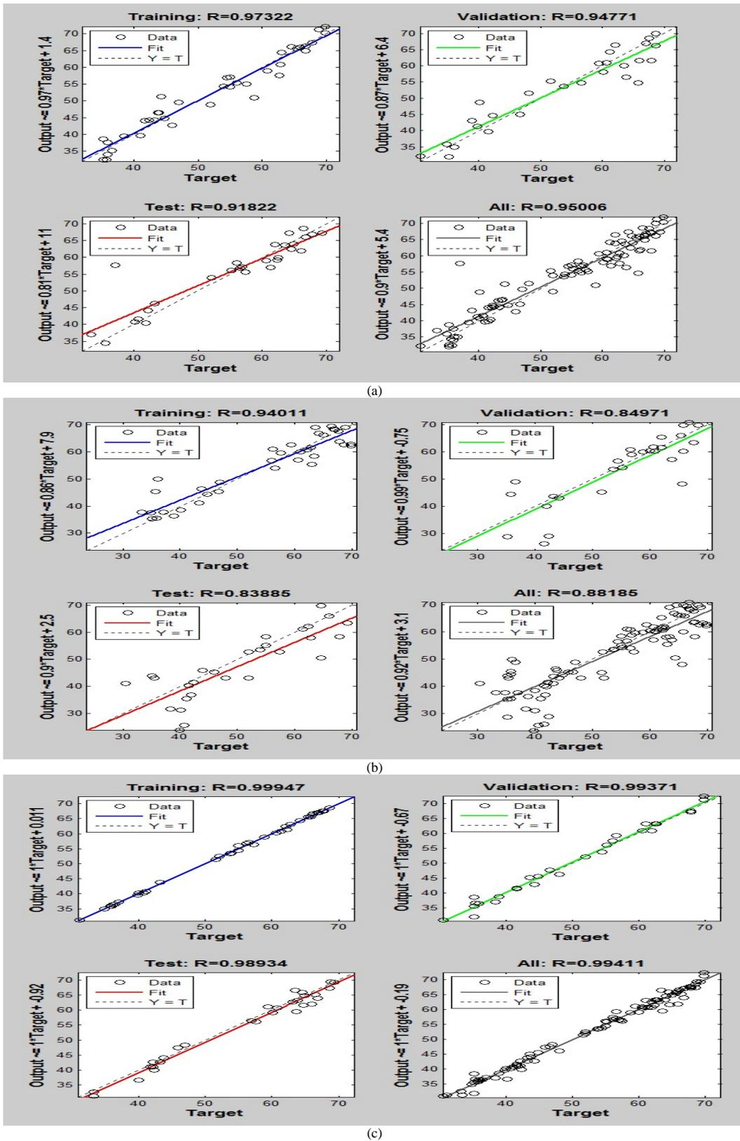
Figure 4: scatter plot of training, validation, test and all data to a) Elman Network b) NARX Network c) Feedforward Network.
