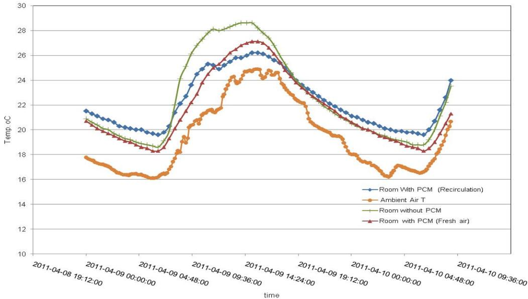
Fig. 14 The indoor air temperatures of the room with and without PCM during a day in spring
