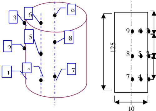
Fig. 5 The PCM Capsule and thermocouple's positions
