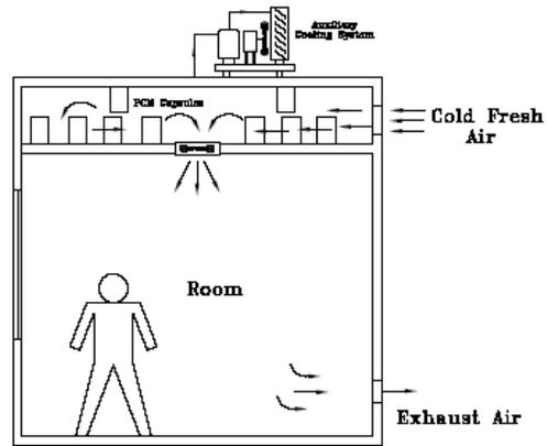
a- PCM capsules cooled at night by fresh air (charge)
