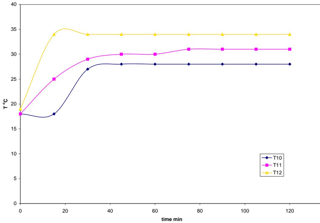
Fig. 11 Air temperature inside the duct
