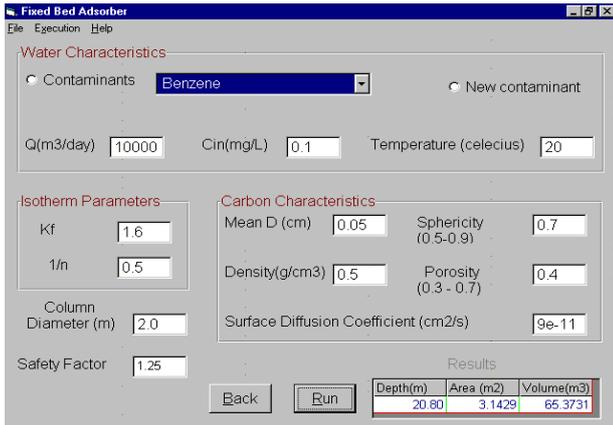
Fig. 5. Fixed bed adsorber window
