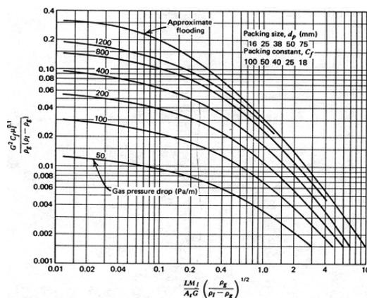
Fig. 3. Flooding and pressure drop correlations for packed towers [14].
