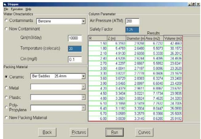
Fig. 4. Air stripper window
