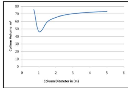
Fig. 8: The relation between FBA volume and its diameter
