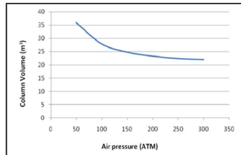
Fig. 9. The relation between AS volume and air pressure
