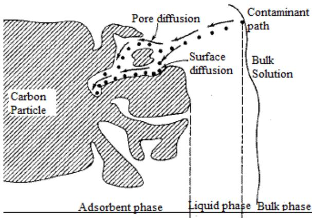
Fig. 1. Adsorption Mechanisms onto GAC [10].
