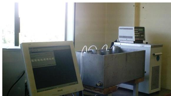
Fig. 1. ANR-100 anaerobic respirometer system.
