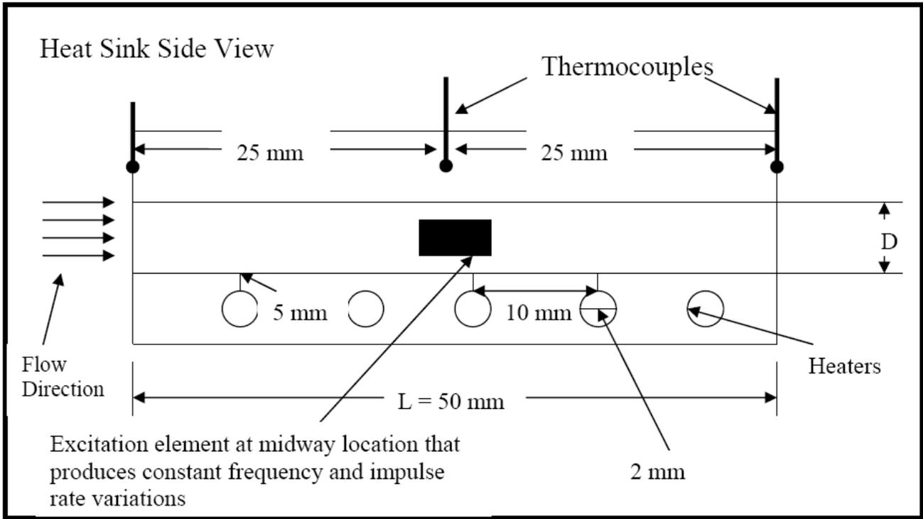
Fig. 2 Detailed schematic of the micro channels
