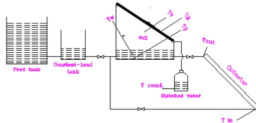
**Fig. 1. Schematic diagram of the active solar still components**
