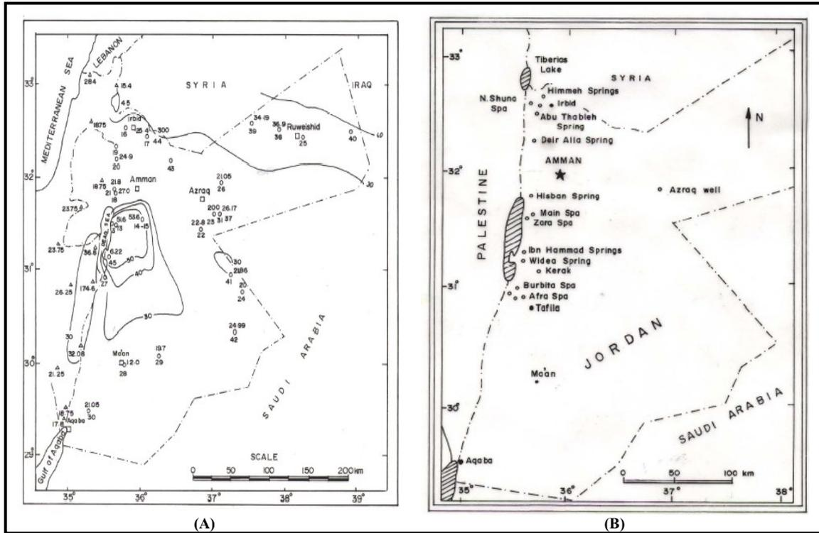
Figure 4. (A) Geothermal gradient map and (B) geothermal resources location map of Jordan [8]
