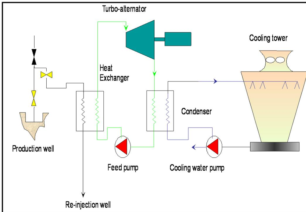
Figure 5. Scheme of the geothermal binary electrical power plant
