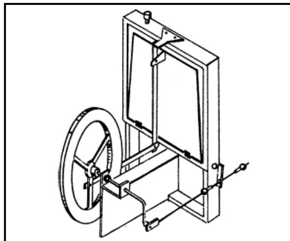
Figure 6. First flat plate low temperature Stirling engine
