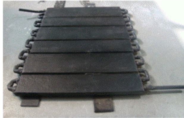
Fig. 6. Casting of solar thermal absorber of 60-40 Cu-Al alloy with copper bends and fittings
