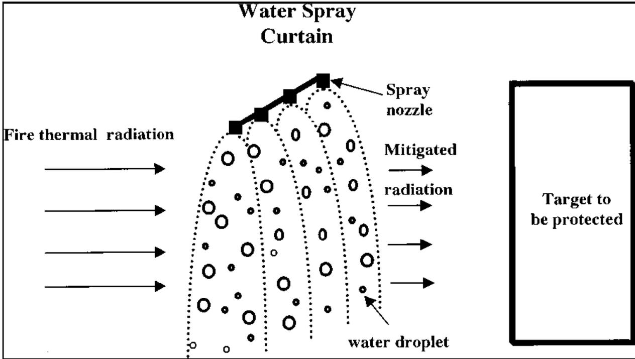
Fig. 1. Water Curtain for Fire protection [4]
