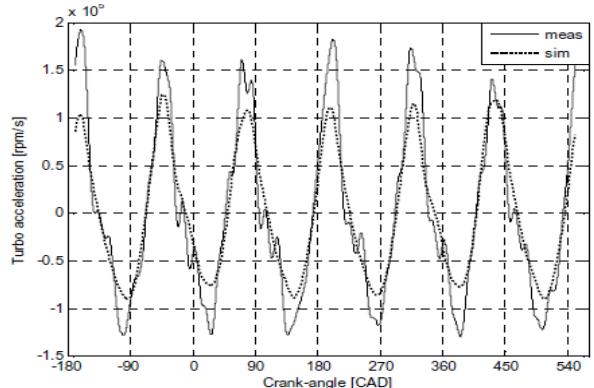
Fig. 15. Comparison between simulated and measured turbo acceleration at different crank angle increments [12]
