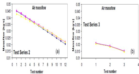
Fig. 13. Comparison between 1D simulation and experimental data from a test. (a) performed with the EGR and throttle valve fully open at 1500 RPM and (b) EGR valve fully open but throttle valve partly open respectively [10]
