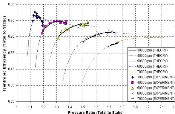
**Fig. 4.** The relationship between the pressure ratio and the isentropic efficiency at varying turbine speeds [2]
