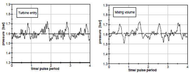
Fig. 3. Variation of pressure at different locations of a turbocharger assembly [1]
