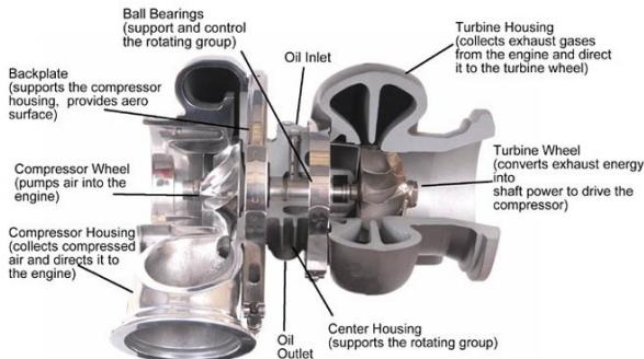
Fig. 1. Typical automotive turbocharger adopting a twin-entry turbine housing ([www.garrett.com](http://www.garrett.com))
