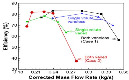
Fig. 12. Efficiency comparisons of the vaneless and vaned single and dual volute designs [9]
