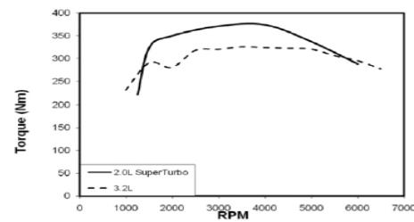
Fig. 18. Comparison of torque between a SI 3.2L NA engine and a 2L SuperTurbo engine over a range of speeds [14]
