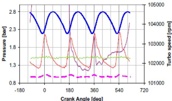
**Fig. 8.** Variation of pressure and turbo speed against crank angle [5]
