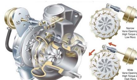
Fig. 19. Variable geometry turbocharger ([www.volvo.com](http://www.volvo.com))
