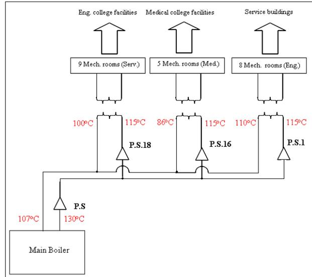
**Fig.10.** Central heating network.
