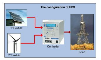
Fig. 1 Configuration of a photovoltaic-wind-grid HPS
