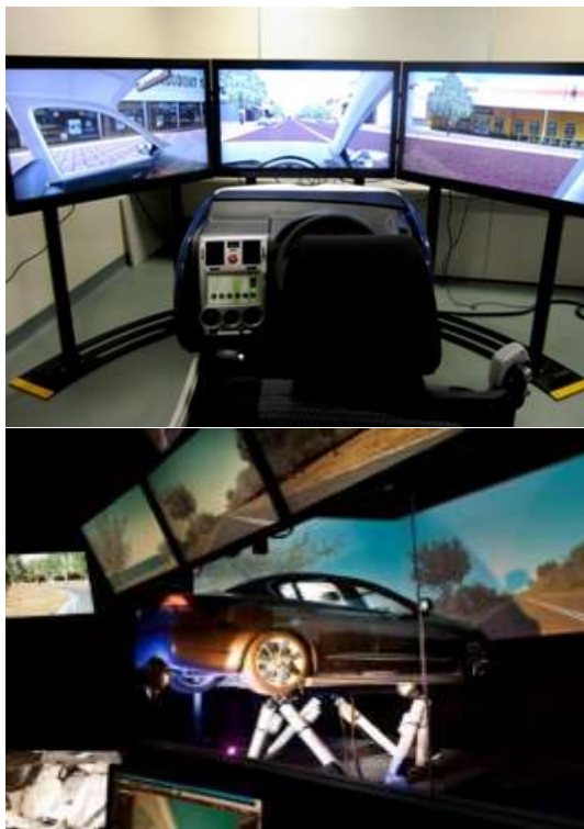
Fig. 1. Fixed Driving Simulator (Up) and Moving Driving Simulator (Down) [21]
