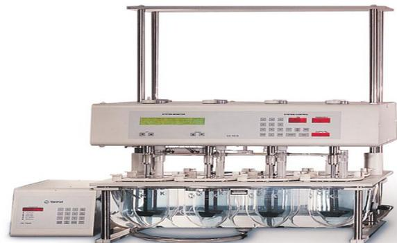
**Figure 1: Varian VK 7010 Dissolution Apparatus that modified as multiple bioreactor.**
