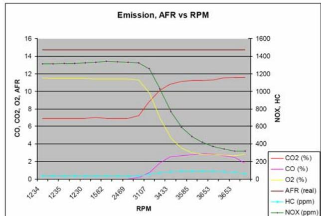
Figure 11: Engine emissions at different RPM - Petroleum Diesel fuel
