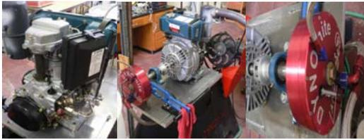
Figure 4: Eight Horse power Diesel Engine and Dynamometer assembly
