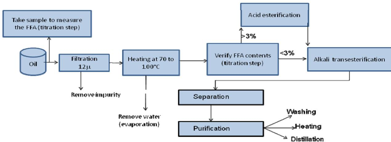
Figure 2: Transesterification following a base catalyst process
