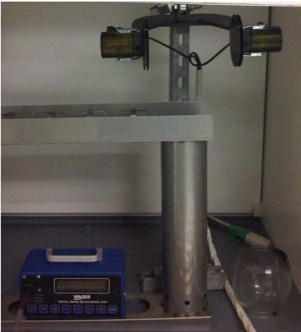
Figure9: Smoke opacity meter experimental set up.
