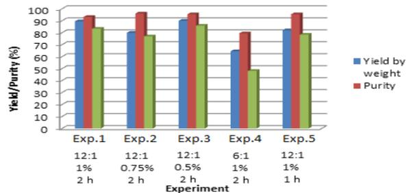
Figure7: WCO biodiesel yield in homogeneous alkaline transesterification at 60°C and continuous stirring.
