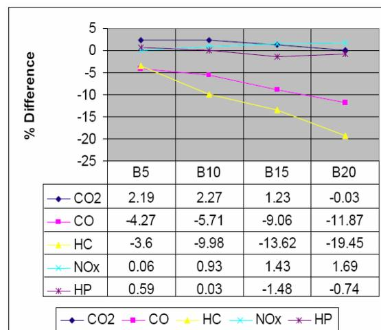
Figure 12: Overall percentage differences of biodiesel fuel blends with respect to petroleum Diesel
