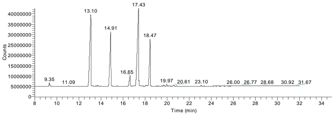
Figure8: Chromatogram of FAME analysis of waste frying oil biodiesel
