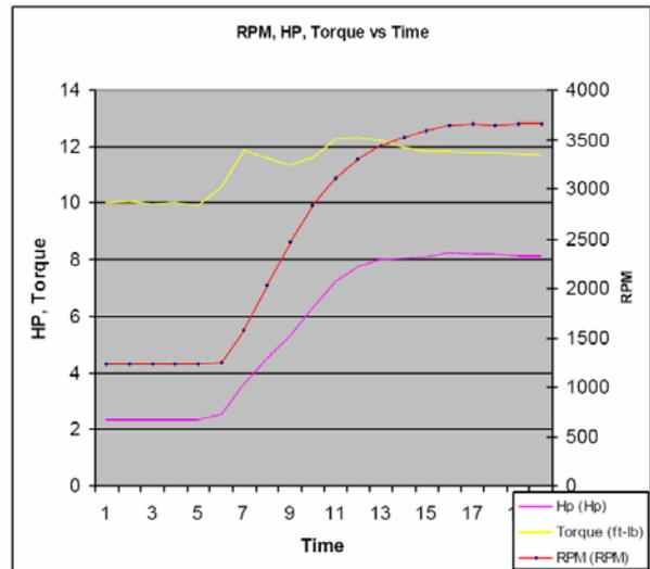
Figure 10: Engine horse power, torque, and RPM versus time (seconds) - Petroleum Diesel fuel
