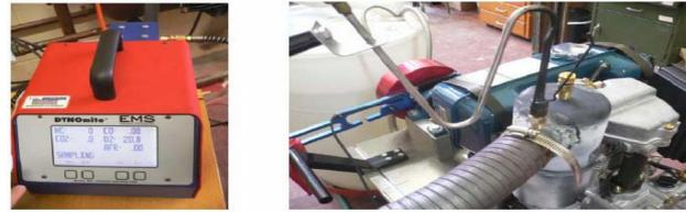
Figure 6: Gas Analyzer
