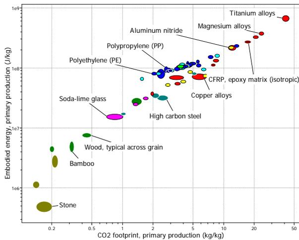
Fig. 2. Embodied Energy and CO<sub>2</sub> footprint for the primary production of materials
