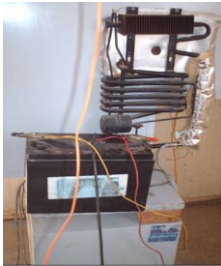
Fig. 12 Solar Absorption Refrigerator
