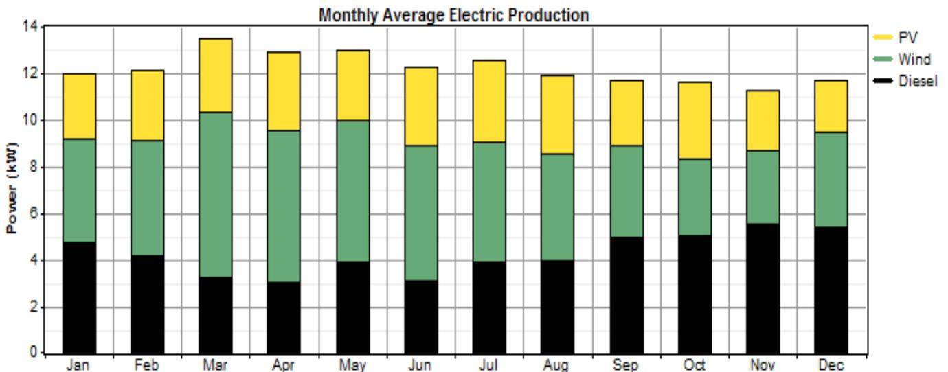
Fig. 7: OPEN-GAIN Burj Cedria site Hybrid system monthly averaged power production
