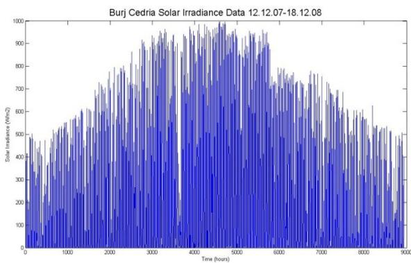
Fig. 5: OPEN-GAIN Burj Cedria site measured hourly solar irradiance data
