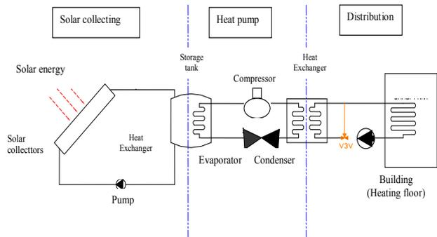
Fig.1. Schematic diagram of solar assisted heat pump system
