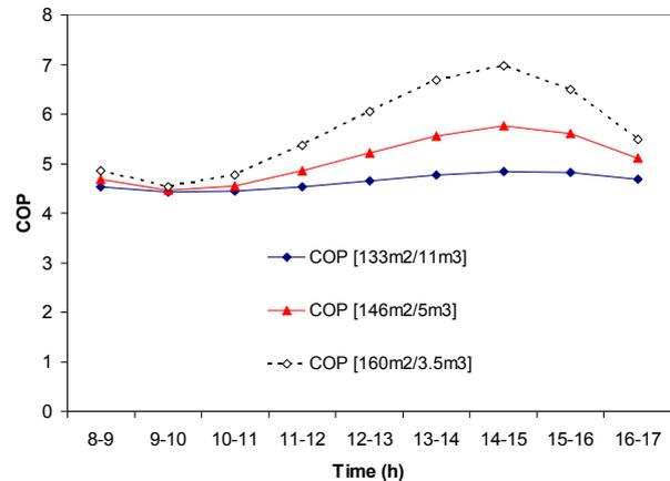
Fig. 3. Variation of the COP versus time of day for various values of the couple  $A_c/V_s$
