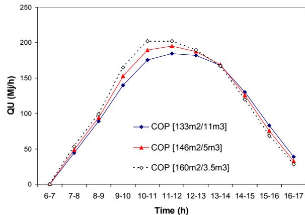
Fig. 4. Variation of the of collected heat versus time of day for various values of the couple  $A_c/V_s$
