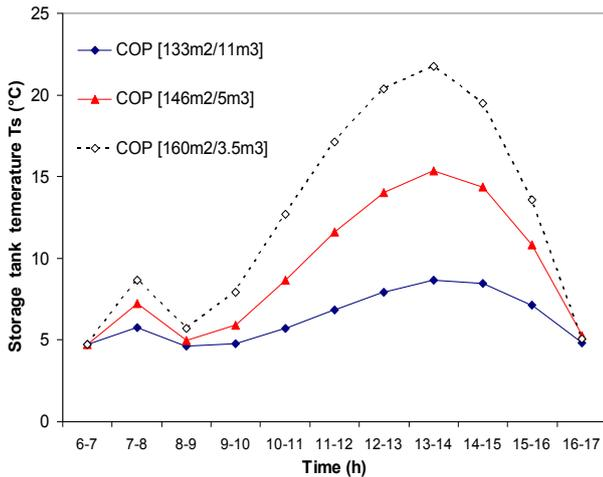
Fig. 5. Variation of the Storage tank temperature versus time of day for various values of the couple  $A_c/V_s$
