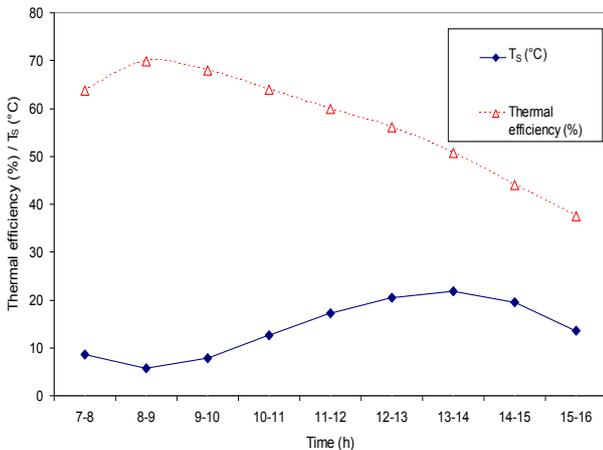
Fig. 6. Variation of the Storage tank temperature and thermal efficiency of solar collectors versus time of day
