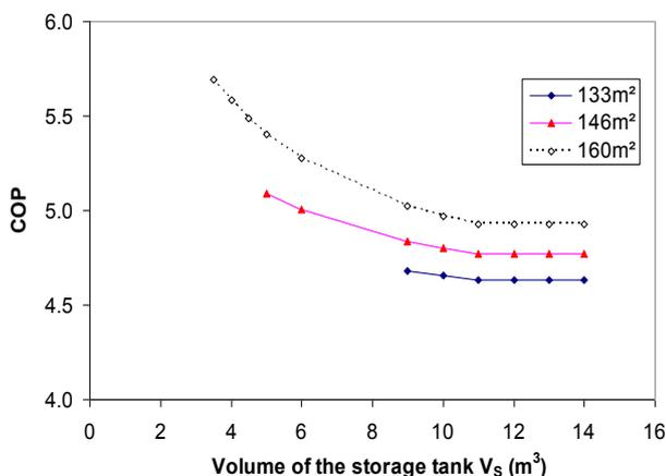
Fig. 2. Variation of the COP versus to the volume of the storage tank ( $V_s$ )
