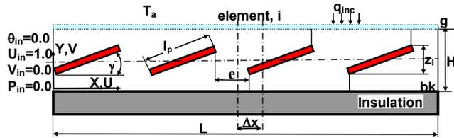
Fig. 2 A schematic diagram for the oblique plates configuration inside the channel
