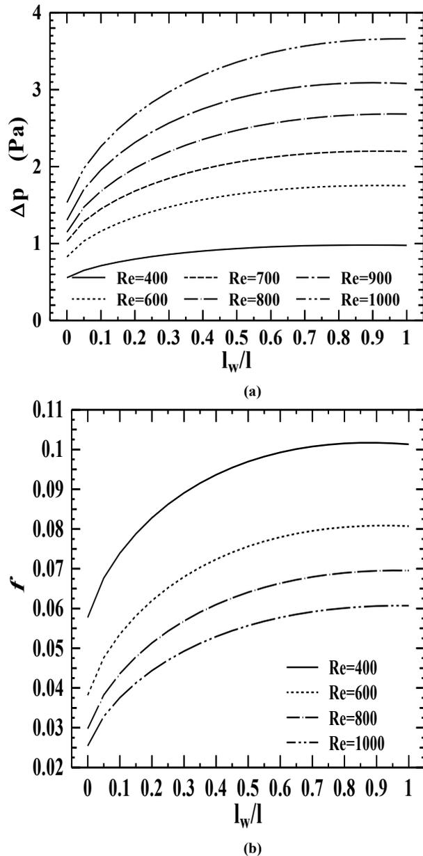
Fig. 4 Effect of plate segments spacing ratio ( $l_w/l$ ) on the total pressure drop and friction factor.
