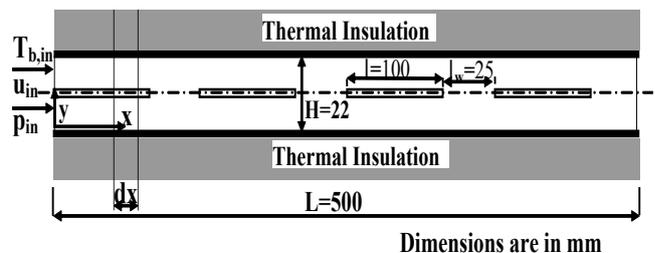
Fig. 1 A schematic diagram for the configuration of the in-line plate segments inside the channel
