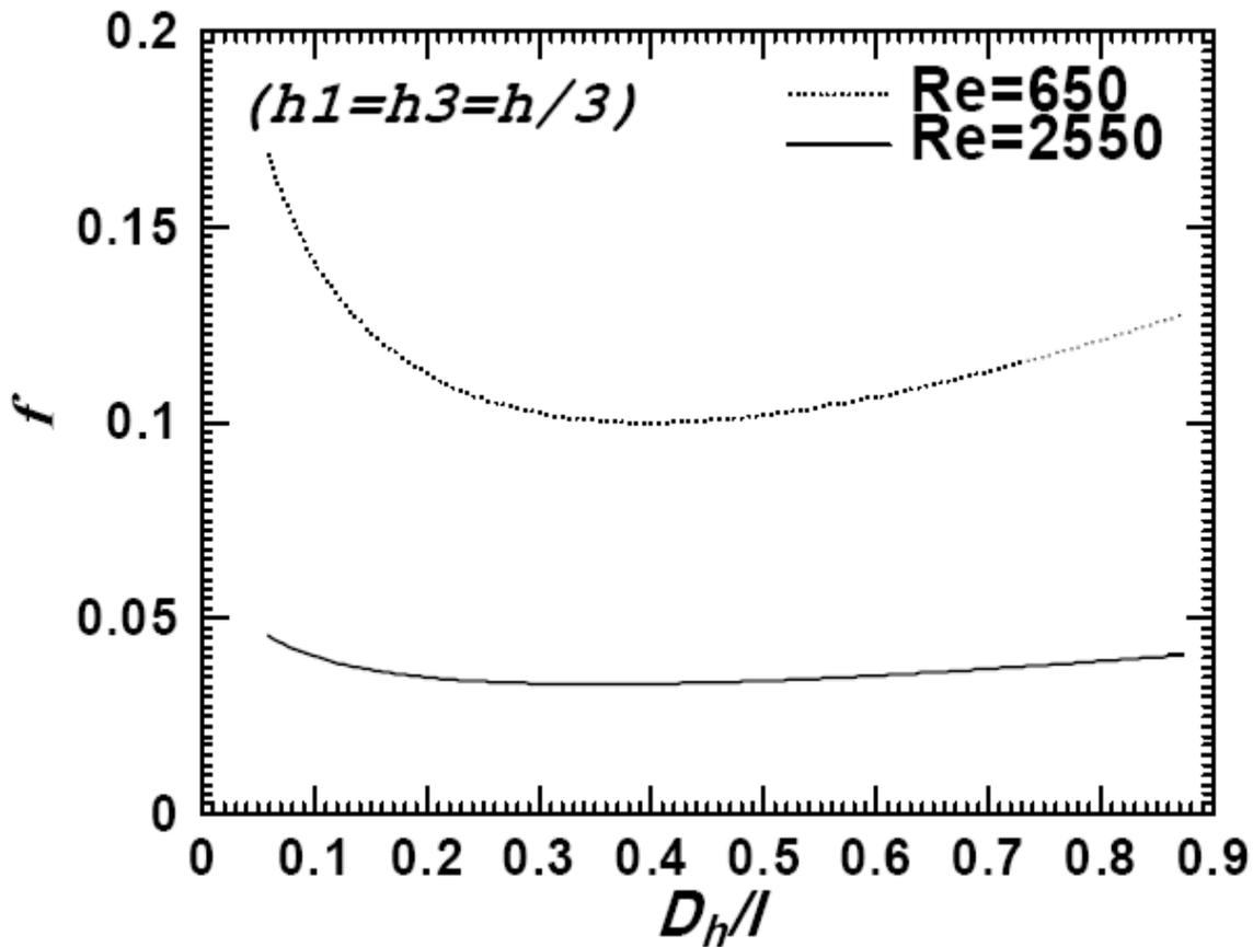
Fig. 7 Effect of the Offset Plate Length on the Friction Factor
