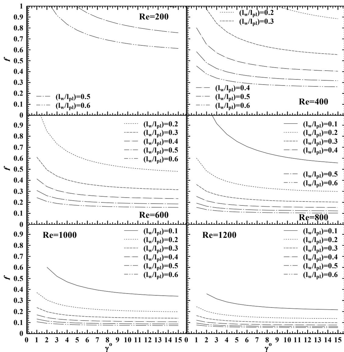
Fig. 6 Effect of plate segments spacing ratio ( $l_w/l$ ) on friction factor
