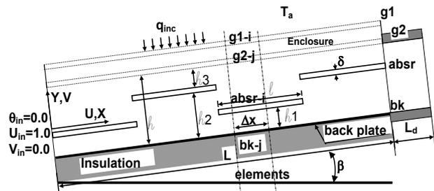
Fig. 3 A schematic diagram for the offset plates configuration inside the channel
