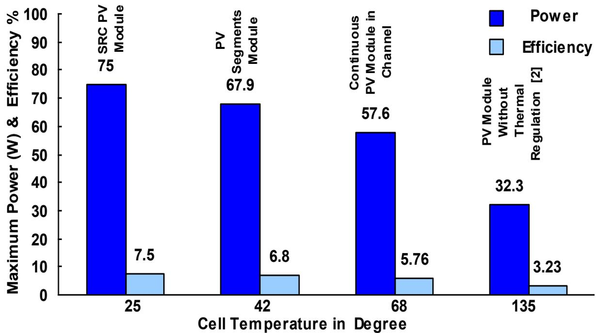
Fig. 8 Comparison of GP 75 PV crystal silicon module characteristics at different operating temperature with those at SRC
