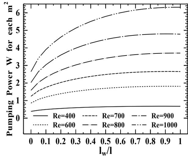
Fig. 5: Effect of plate segments spacing on the pumping power
