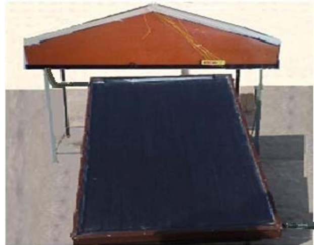
Fig.2. Photograph of double slope active solar still set up
