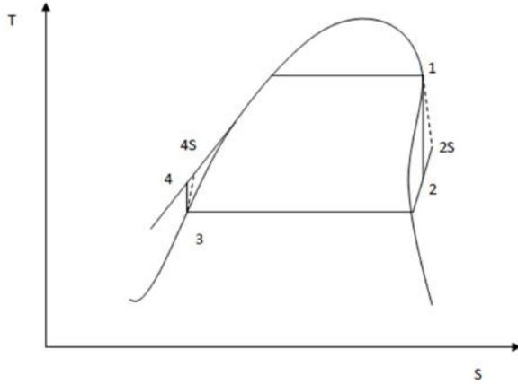
Fig. 1. T-S diagram of ORC with dry refrigerant and saturated vapor at turbine inlet
