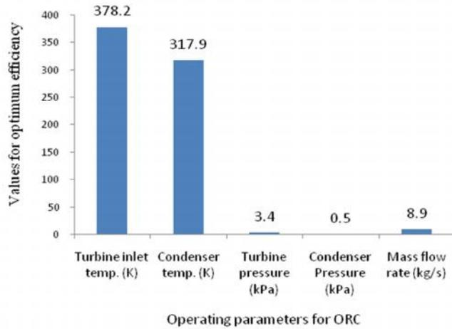
d. Chart depicting the values of operating parameters for maximum thermal efficiency output for R-123
