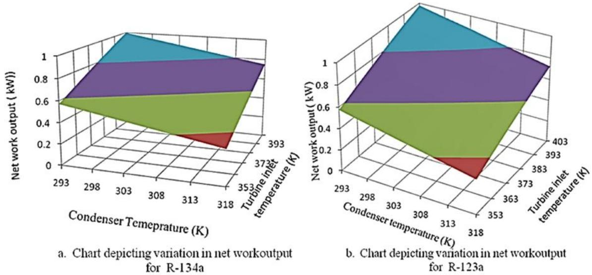
Fig.6. Net work out put verses condenser temperature and turbine inlet temperature
