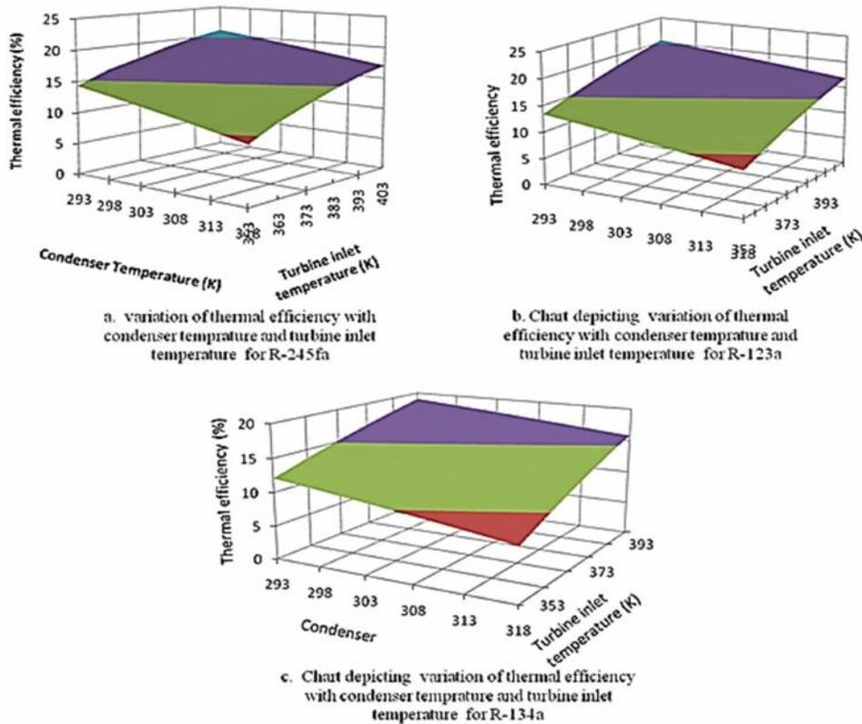
Fig. 5. Thermal efficiency verses condenser temperature and turbine inlet temperature
