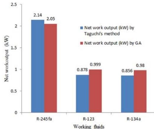
Fig. 7. Comparison of optimum Net workoutput of ORC estimated by Taguchi's method and genetic algorithm
