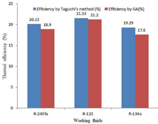
Fig. 8. Comparison of optimum thermal efficiencies of ORC estimated by Taguchi's method and genetic algorithms
