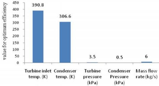
b. Chart depicting the values of operating parameters for maximum thermal efficiency for R-245fa
