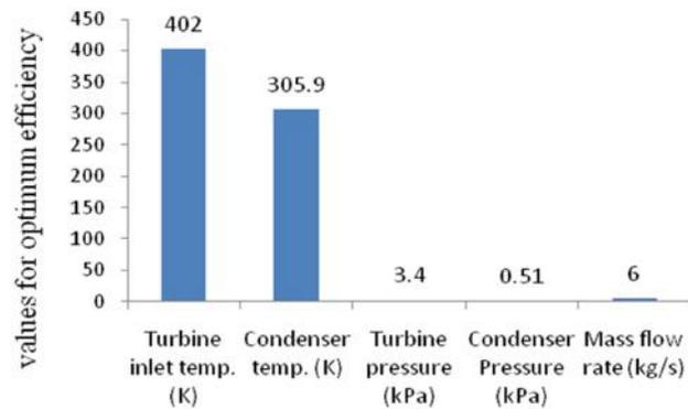
f. Chart depicting the values of operating parameters for maximum thermal efficiency for R-134a
