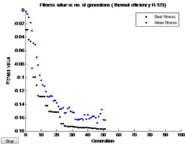
c. Fitness value vs number of generations for thermal efficiency using R-123
