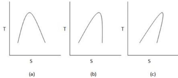
Fig. 2. Different types of working fluids (a) wet, (b) isentropic and (c) dry
