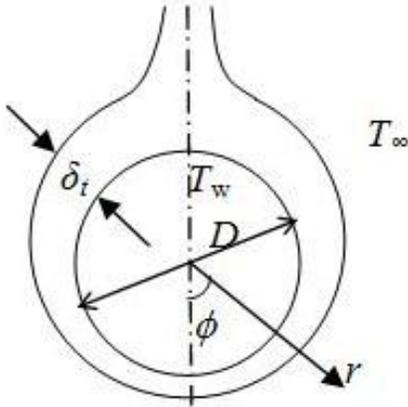
Figure 2. Schematic diagram of a horizontal solid cylinder immersed in stagnant air
