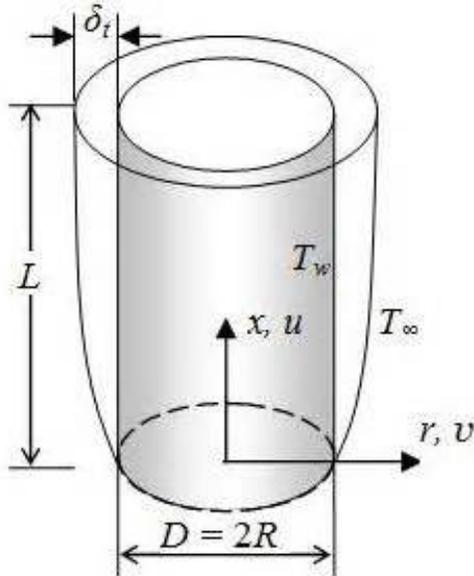
Figure 1. Schematic diagram of a vertical solid cylinder immersed in stagnant air
