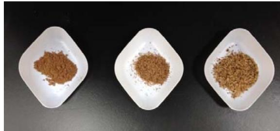
**Figure 2: Samples of Khalas date seed with sizes adjusted in the ranges of 0.425 – 0.6 mm, 0.6 – 1.18 mm, and 1.18 – 3.75 mm**
