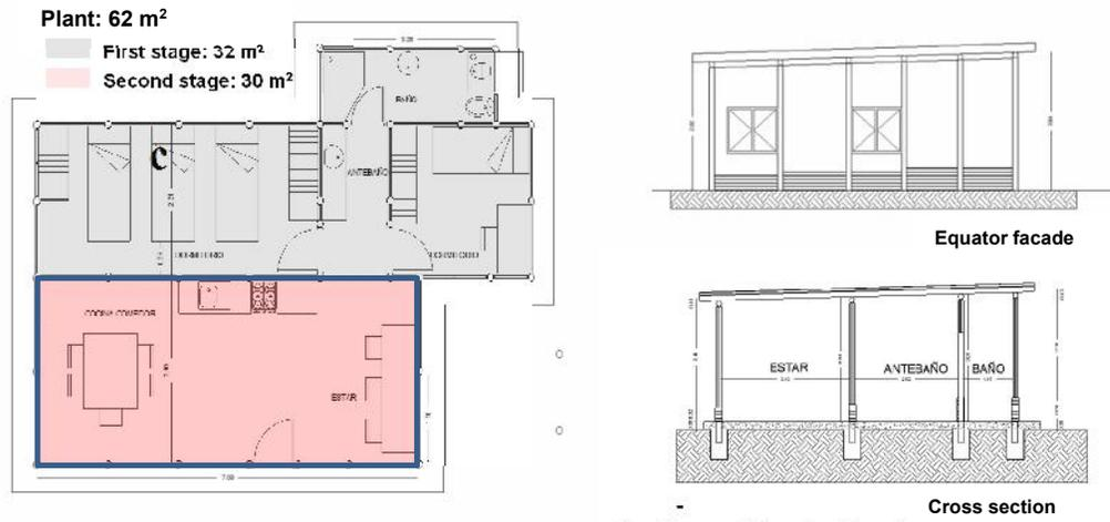
Figure 3: Plants of 1° and 2° Stage, Cross Section and Equator Facade.
