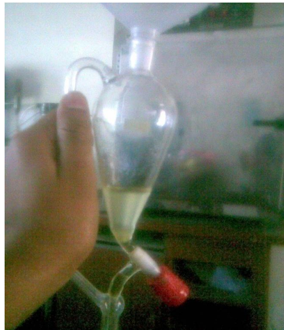
Fig. 4 Upper layer of esters and lower of potassium hydroxide solution
