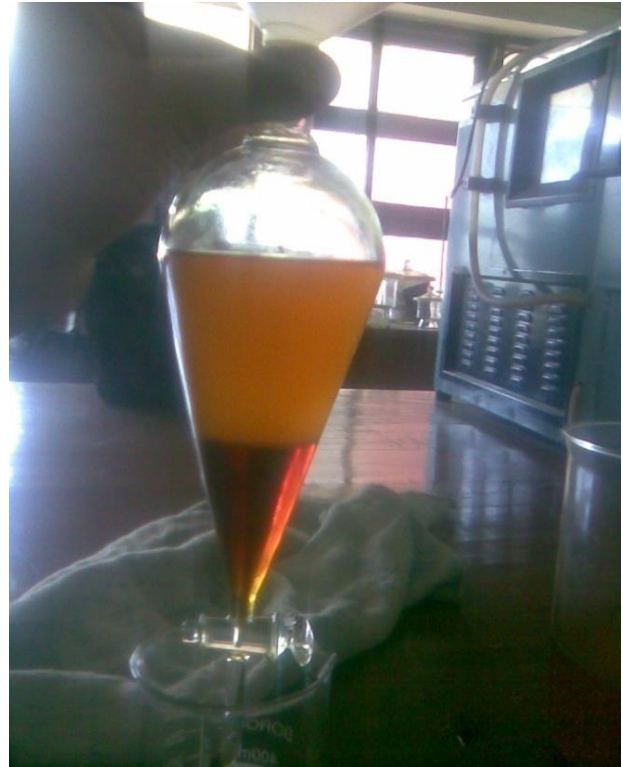
Fig. 3 Upper layer of bio-fuel and lower layer of glycerol
