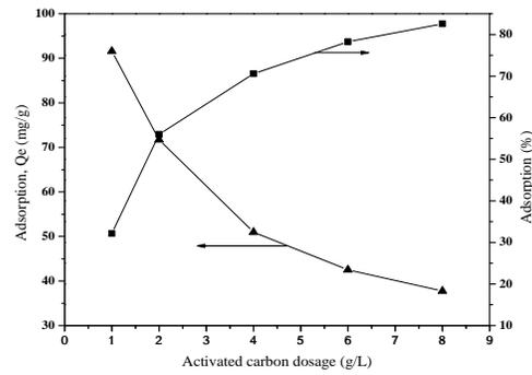
Figure 6: Effect of ACG dosage on adsorption of phenol [C<sub>0</sub> = 150 mg.L<sup>-1</sup>, ACG dosage 1-8 g.L<sup>-1</sup>, adsorption time: 24 h, Adsorption, Q<sub>e</sub>; Adsorption (%)]
