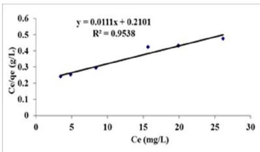
**Figure 8B: 1st order Kinetic Model of Phenol Adsorption on ACG**
