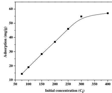
Figure 7 Influence of Initial Phenol Concentration C<sub>0</sub> on ACG [C<sub>0</sub> = (75 – 300) mg.L<sup>-1</sup>, ACG Loading: 5 g.L<sup>-1</sup>, Adsorption Time: 16 h];
