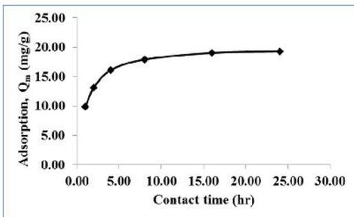
**Figure 8A: Effect of Contact Time on Phenol Adsorption by ACG**
