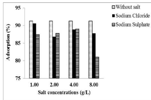
**Figure 9: Influence of Two Salts on the Adsorption of Phenol by ACG (Phenol Conc: 300 mg/L, ACG dosage: 5 g/L, Adsorption Time: 16 h)**
