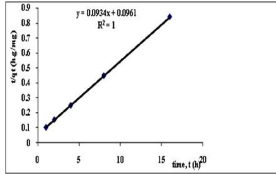
**Figure 8C: 2<sup>nd</sup> Order Kinetic Model of Phenol Adsorption on ACG**
