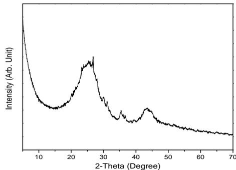
Figure 2: XRD Pattern of Original Activated Carbon Granules
