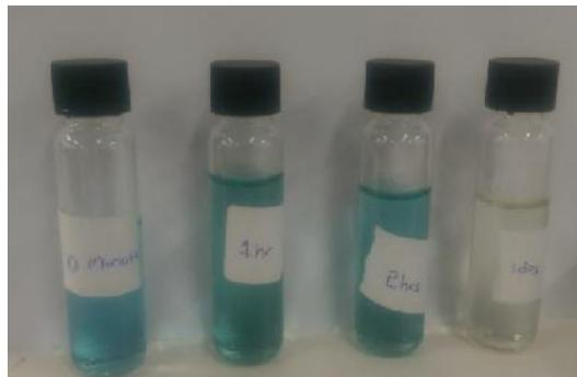
Figure 6: Color Change of the Refinery Cooling Water after UV Treatment
