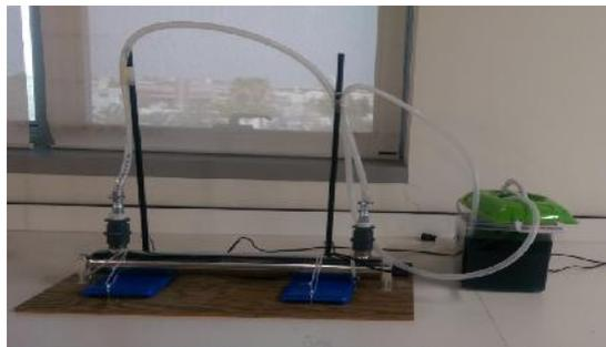
**Figure 1: Bench Scale UV-Reactor for a Cooling Water Recirculating System**
